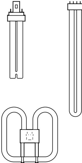
Compact fluorescent lamps (CFLs) have the characteristics and advantages of linear fluorescent lamps, but with compact size. Lamp designers have been able to fold the discharge path while retaining high efficacy. The phosphors used are triphosphors. New lamps are frequently introduced, and it is essential to consult the catalogues of LIF lamp manufacturers. This Guide explains the variety of CFLs. The two main groups are: CFLs – External Control Gear, and CFLs – Integral Control Gear.
