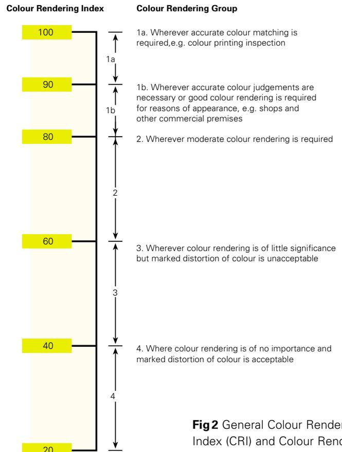
**Fig 2** General Colour Rendering Index (CRI) and Colour Rendering Groups for typical applications.
