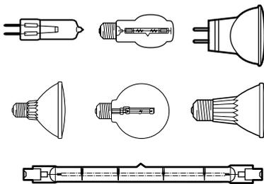
These are filament lamps with a halogen (added to the gas filling), which prevents evaporated tungsten blackening the bulb. Tungsten Halogen lamps have an increased light output and/or extended life compared with standard filament lamps. The bulb is of small dimensions, and made from quartz or hard glass. Some mains voltage lamps have an outer bulb.
