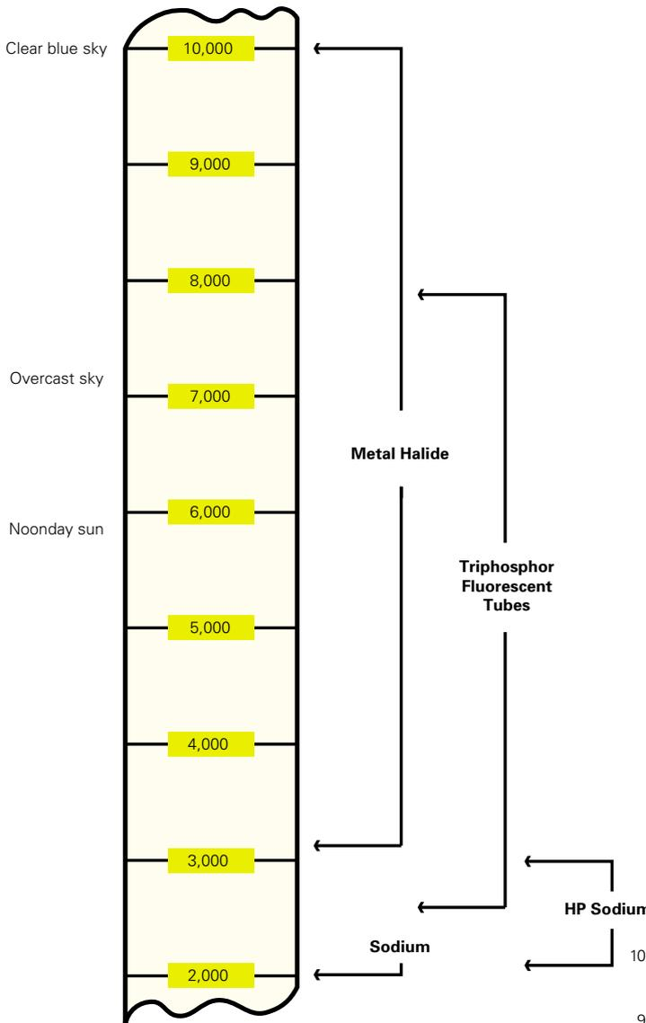
**Fig 1** Correlated Colour Temperature (CCT) for some lamps
