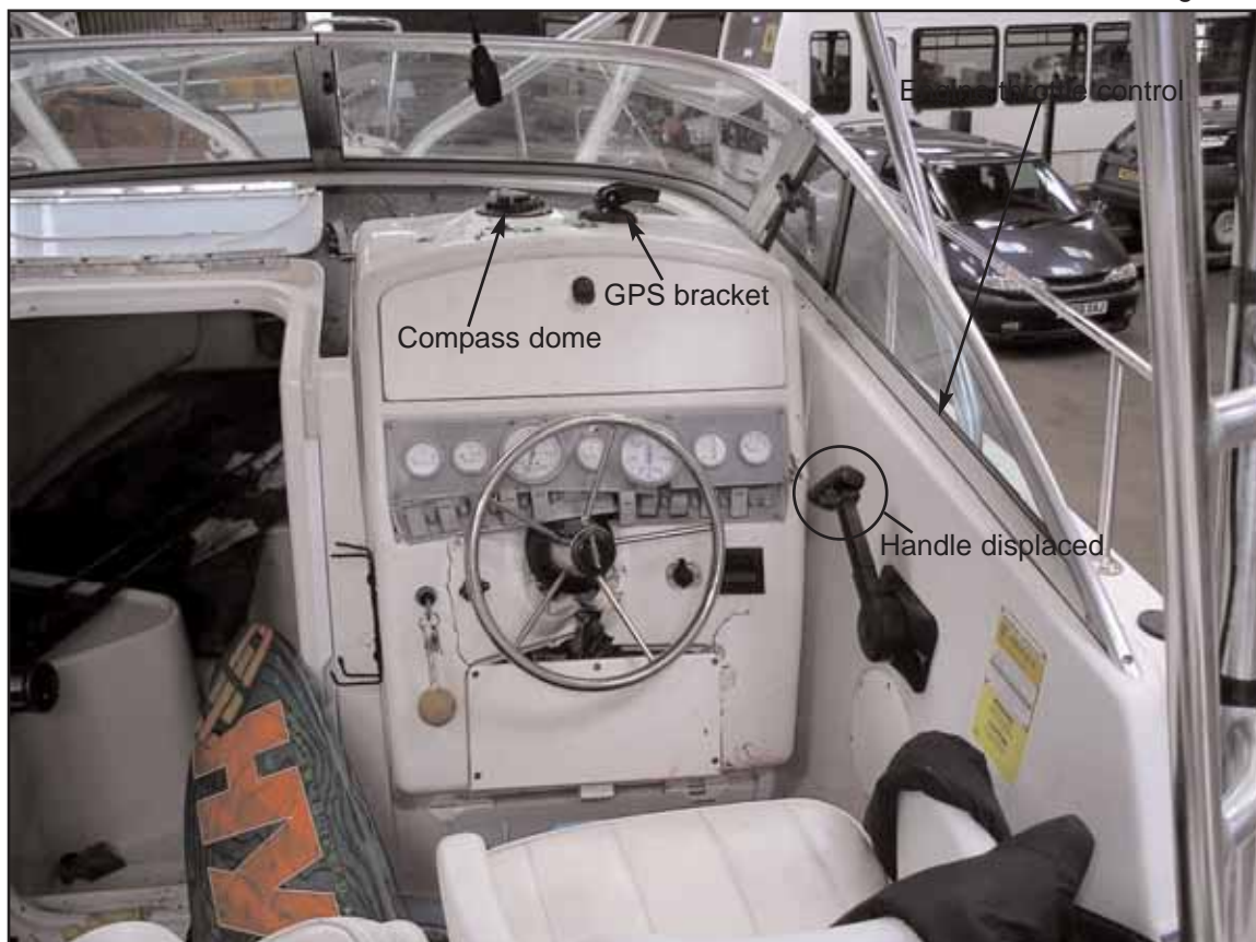
A photograph of the cockpit area showing damage to instrument panel, the engine throttle control lever and the companionway door
