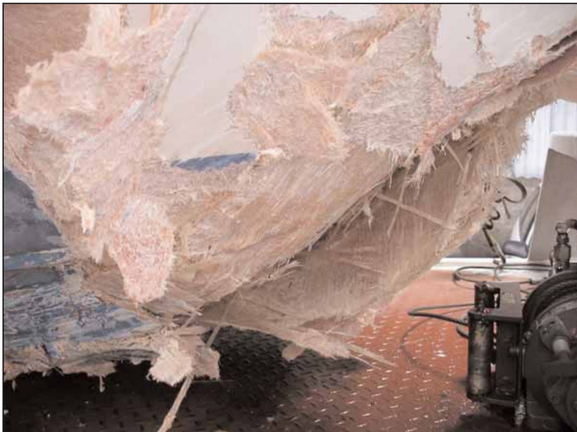
Looking at the damage to starboard forefoot and bow forward
